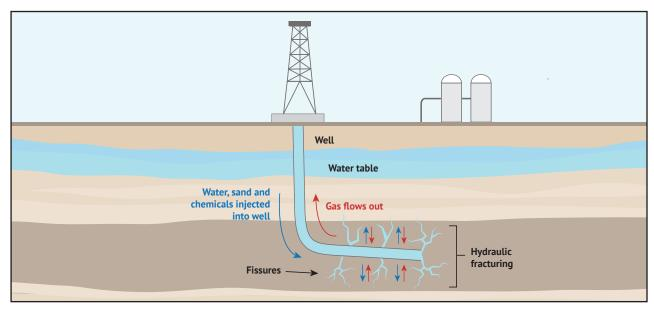
Shale gas extraction. https://www.consumernotice.org/environmental/fracking/ (modified)
